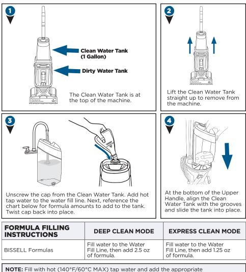
**NOTE:** Fill with hot (140°F/60°C MAX) tap water and add the appropriate BISSELL formula. **DO NOT USE BOILING WATER. DO NOT HEAT WATER OR TANK IN MICROWAVE.** Do not substitute BISSELL Formula with other household cleaning products.
