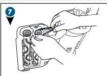
To replace the cogged large pump belt, make sure your deep cleaner is completely reclined. Begin by wrapping the cogged large pump belt around the small metal-toothed pulley. While wrapped around the pulley, stretch and wrap around the nearest brush gear.
