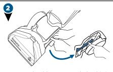
Here you should see one (1) belt. This is the flat pump belt. If this belt is broken, gently remove it from the machine. We will replace this belt in Step 5.
