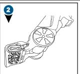
Lay the machine down on its back or side.
