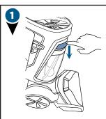
To release Dirty Water Tank, press down on the colored tank handle.
