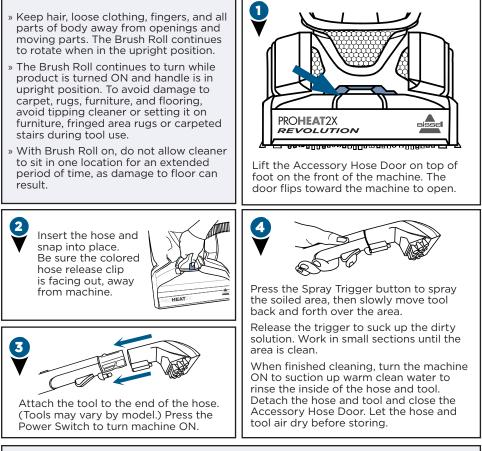
**NOTE:** If using the **Mini Deep Reach Tool**, be sure the needles of the tool are pressed down into the carpet so the spray gets into the carpet fibers.
